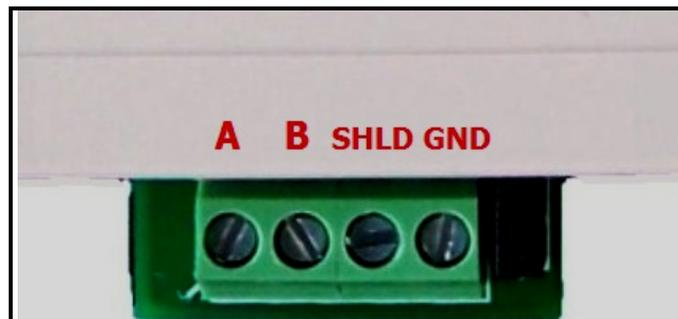
Figure 9: RS-485 Connection Terminals
