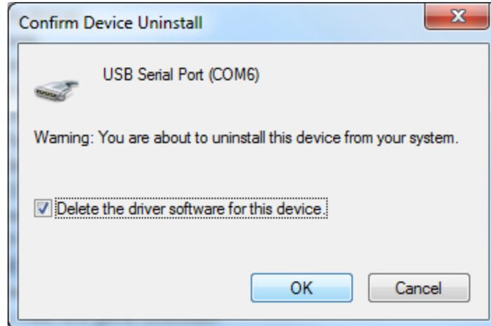
Figure 8: Uninstall comport to release assigned number
